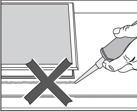
The sealing strip under the edge of the upper part of the cooktop provides an adequate seal against the countertop.
